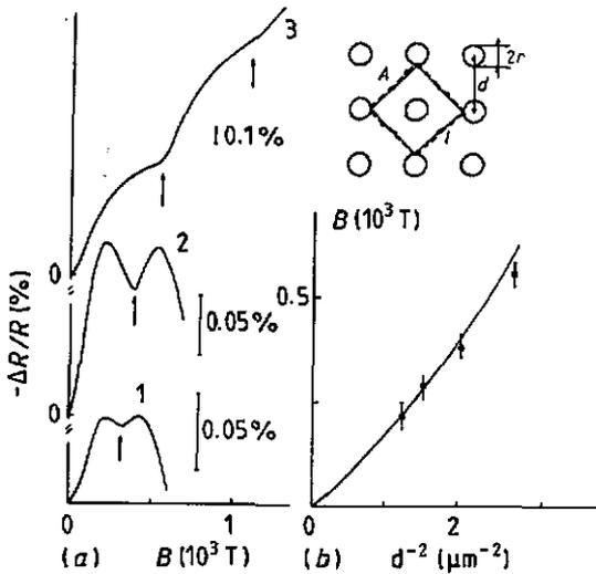
**Figure 2.** (a) Low-field dependence of the resistance on  $B$  for samples with different lattice periods  $d$ : (1)  $0.8 \mu\text{m}$ , (2)  $0.7 \mu\text{m}$ , (3)  $0.6 \mu\text{m}$ ;  $T = 1.7$  K. (b) Period of low-field oscillations as a function of  $d^{-2}$ . The solid curve is given by  $B_0 = hc/e\ell^2$ . Insert—sketch of the electron trajectories contributing to Aharonov-Bohm oscillations.
