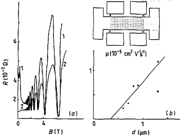
Figure 1. (a) Magnetoresistance in patterned (1) and bare samples (2).  $T = 4.2$  K; lattice period (patterned sample)  $d = 0.9 \mu\text{m}$ . (b) Mobility of the patterned samples as a function of period  $d$  (open circle, sample with elliptical shapes of imposed scatterers). Insert—sketch of the sample geometry.
