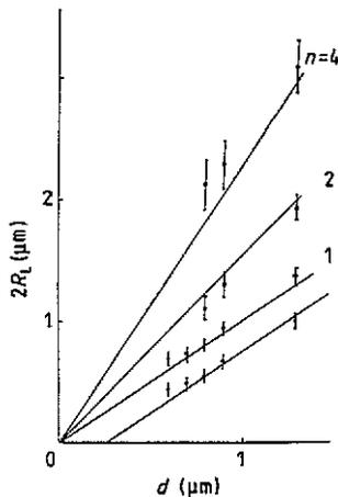
Figure 4. Cyclotron diameter in the peaks of oscillations as a function of  $d$ . The solid line is given by: (1)  $2R_L = d$ , (2)  $2R_L = 1.6d$ , (4)  $2R_L = 2.28d$ , where  $n$  is the number of antidots corresponding to a pinned orbit. Bottom line— $2R_L = d - c$ .
