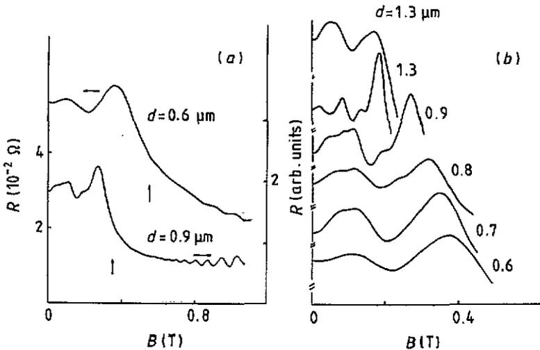
Figure 3. (a) Commensurability oscillations and negative magnetoresistance for two samples with different periods  $d$ . Arrows indicate the features in the negative magnetoresistance curve. (b) Magnetoresistance oscillations from samples with different lattice periods. Top curve—sample with elliptical shaped scatterers of length  $0.6 \mu\text{m}$  and width  $0.2 \mu\text{m}$ ; other curves—samples with hole-shaped scatterers of diameter  $2r = 0.2 \mu\text{m}$ .
